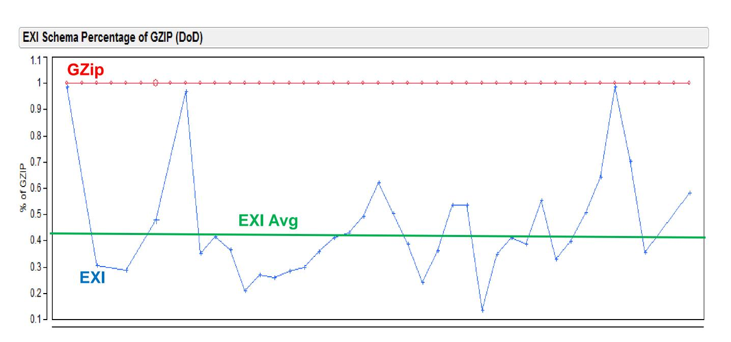
EXI compared to GZip (standard compression) in the long run average is 42% of GZip = 116% increase in bandwidth potential for DoD
